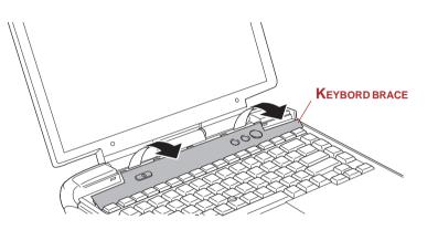
Figure 8-7 Removing the keyboard brace
